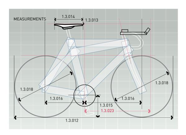
The profile of the extension must conform to the 1:3 ratio in accordance with Article 1.3.024. The extension must be fixed and not feature a system that would allow a change of length or angle during the race.
